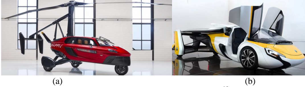
Fig. 3: Examples of flying cars: (a) VTOL designed by PAL-V 10 , (b) STOL designed by Aeromobil 11
